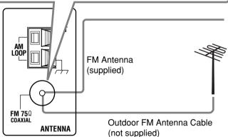
Connect the supplied FM antenna as temporary measure to the FM 75  $\Omega$  COAXIAL terminal—
